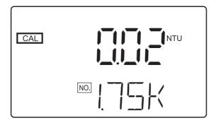
8 Insert the 1750 NTU calibration standard into the cuvette shaft.
