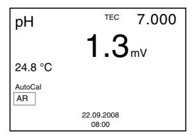
Wait for the measurement with stability control to be completed or terminate the stability control and take over the calibration value with **<ENTER>**.
