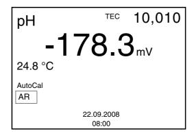
18 Use **<M>** to finish calibration or switch to calibration with the next buffer with **<ENTER>**.
