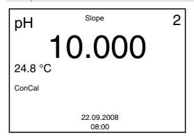
Take over the calibration value for the slope with **<ENTER>**. The calibration is completed as a two-point calibration. The calibration record is displayed.
