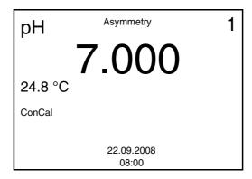
Wait for the measurement with stability control to be completed.
