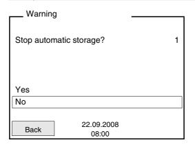
2 Using <▲><▼>, select Yes and confirm with <ENTER>. The meter switches to the measured value display. The automatic storage function is terminated.
