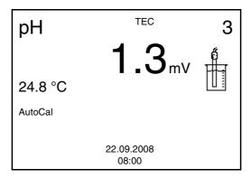
If necessary, terminate the calibration as a two-point calibration with <**M**>.
