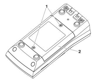
Place four batteries (type Mignon AA) in the battery compartment.
