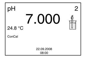
If necessary, terminate the calibration as a single-point calibration with <M>.
