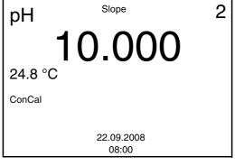
15 Take over the calibration value for the slope with **<ENTER>**. The calibration is completed as a two-point calibration. The calibration record is displayed.
