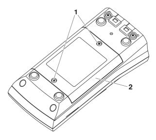
3 Place four batteries (type Mignon AA) in the battery compartment.
