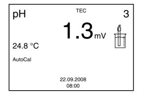
13 If necessary, terminate the calibration as a two-point calibration with <M>.
