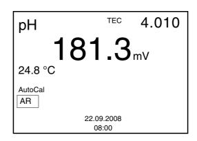
6 Wait for the end of the measurement with stability control or accept the calibration value with <ENTER>.
