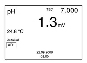
12 Wait for the measurement with stability control to be completed or terminate the stability control and take over the calibration value with **<ENTER>**.
