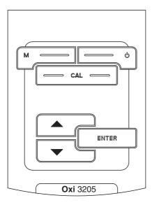
In this operating manual, keys are indicated by brackets <..> . The key symbol (e.g. **<ENTER>**) generally indicates a short keystroke (under 2 sec) in this operating manual. A long keystroke (approx. 2 sec) is indicated by the underscore behind the key symbol (e.g. **<ENTER\_\_**>).
