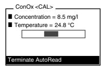
Wait for the end of the AutoRead measurement or accept the measured value with <MENU/ENTER>.
