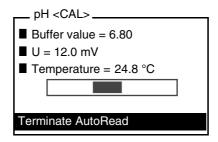
8 Wait for the end of the AutoRead measurement or *Terminate AutoRead* and accept the calibration value with <meNU/ENTER>.
