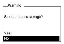
Select and confirm Yes with <**△>** <**▼>** and <**MENU/ENTER>**. The measuring instrument switches to the measured value display.
